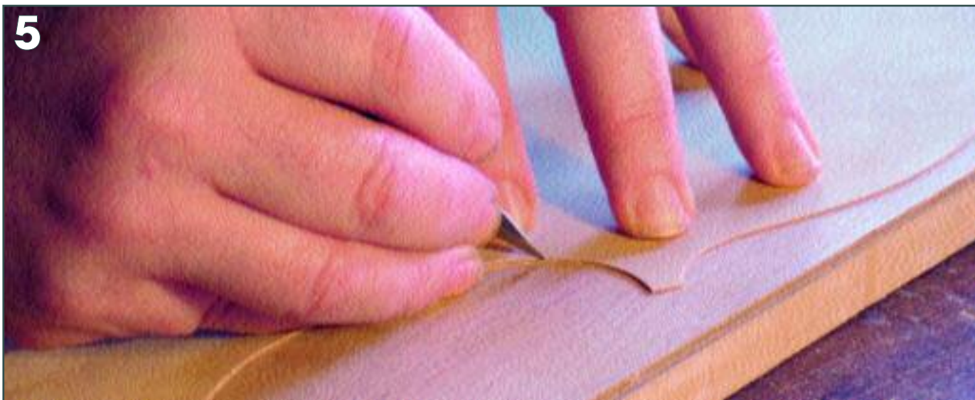
Trace round the outer template with a sharp knife, marking the inner template beneath it
