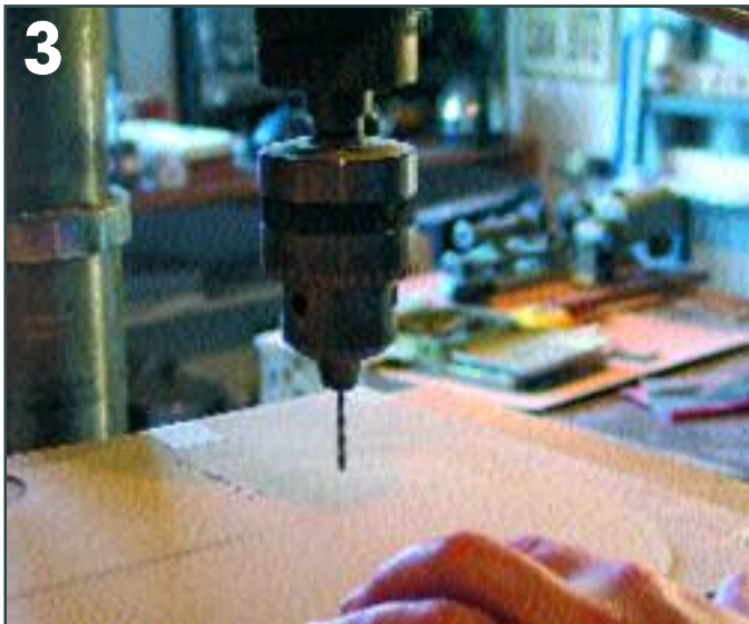
Tape the templates together and drill the positioning holes
