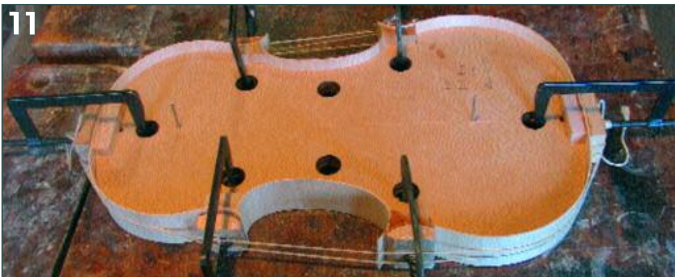
Have the nylon cord handy when you're fixing the ribs
