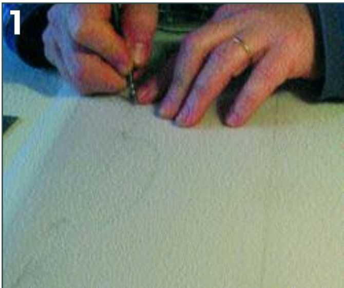
Prick the outline of the instrument through the drawing on to the plywood
